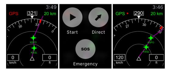
Figure 6.1: flyNav Watch App. Left hand side: Initial navigation screen with deactivated navigation. Middle: Navigation menu after making a force touch on the display. Right hand side: Started navigation.
