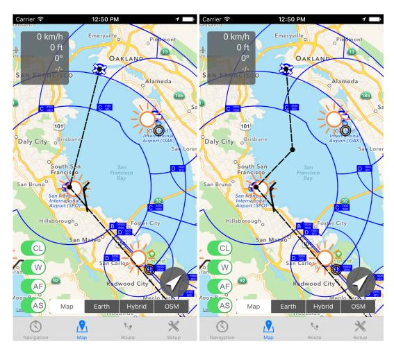
Figure 4.2: A planned route. Left hand side: Route with two waypoints (departing airport and destination airport). Right hand side: A route with an inserted free GPS-waypoint.
